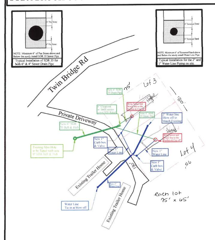
NOTE: ALL ABOVE DRAWINGS ARE NOT TO SCALE Proposed New Sewer Lines and Water Lines for Lot #3 and Lot #4 39 Twin Bridge Rd. Tilton, New Hampshire 03276
